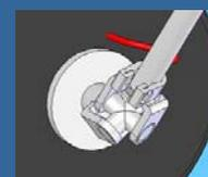
The ball-and-socket joints attach the suction pads to the structure in a flexible manner, permitting rotation with two degrees of freedom in the case of our device.
