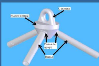
**Eyebolt:** This part is screwed securely to the core unit.
