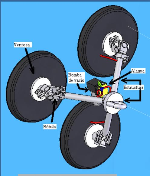
Anchoring device structure
